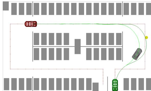
Fig. 1. Motion planning for navigating through a car park. Start (green frame), goal (red frame), prior knowledge of static obstacles (grey) and a roadmap (red) are provided. The initial result from SEHS engine (dark green line) is adapted (light green line) after detecting an obstacle (yellow).
