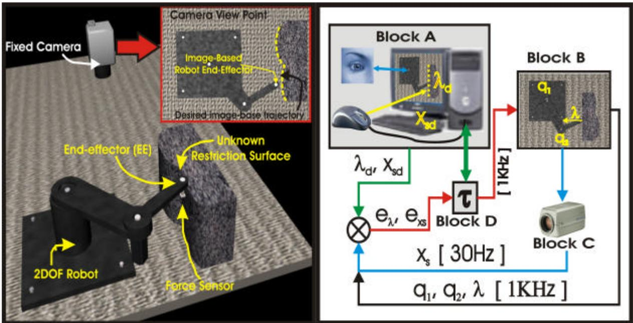
Figure 1. Robot Force-Vision Experimental System: Where,  $e_\lambda$ ,  $e_{x_s}$ , stands for force errors and visual errors.  $l_d$  is the desired force,  $l$  is the applied end effector force,  $x_s$  is the visual position of the robot end-effector and  $q_i$ , stands for generalized position. The Restriction Surface is unknown but with continuous gradient.
