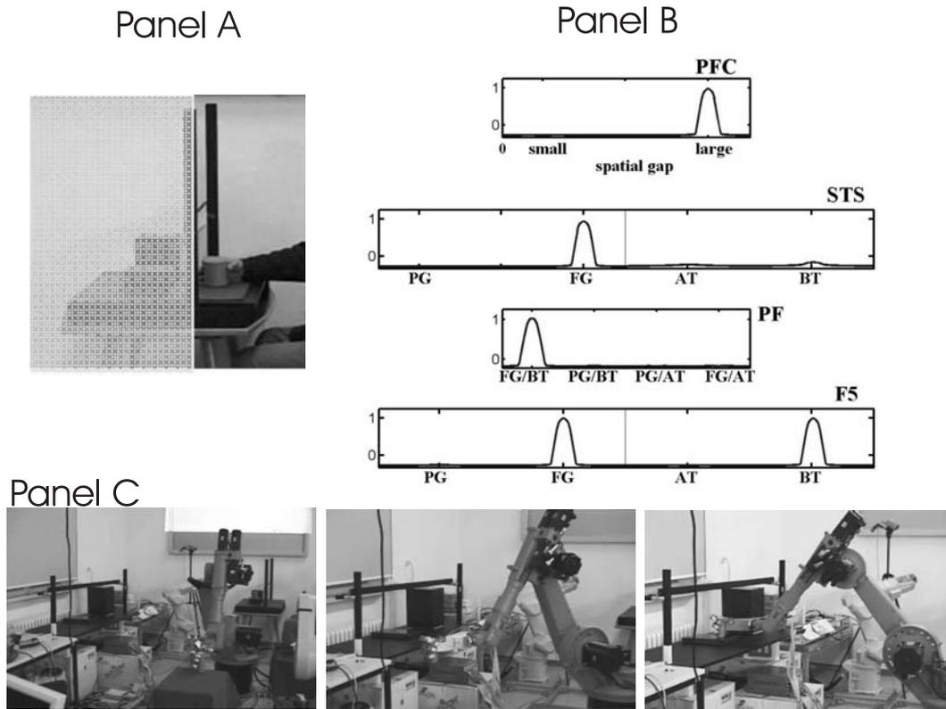
Fig. 4. Inference task. **Panel A:** Only the grasping behavior is observable. **Panel B:** The stable state in layer PFC of the field model represents the inferred goal (here lower goal). **Panel C:** To reproduce the inferred end state the robot combines a full grip (FG) followed by a trajectory below (BT) the bridge as represented in the motor layer F5 in Panel B.
