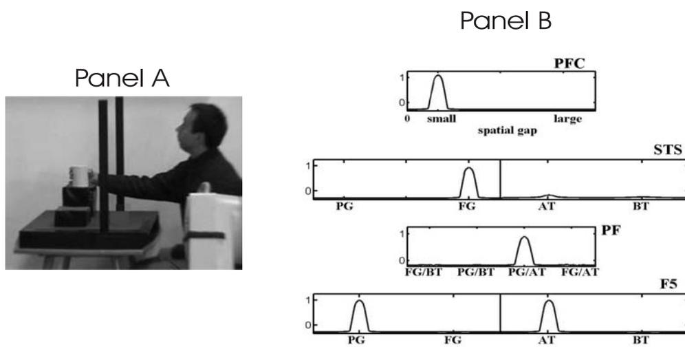
Fig. 5. Goal directed imitation. **Panel A:** Conflict in the grasping behavior, i.e. the teacher uses a full grip for placing the object in the higher goal position. **Panel B:** As shown in layer F5 of the field model, the robot decides to use a precision grip to reproduce the observed end-state.
