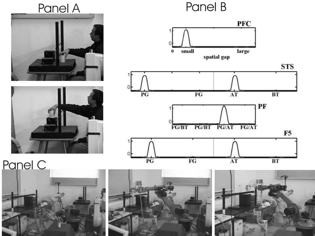
Fig. 3. Copying the means. **Panel A:** The teacher shows a complete grasping-placing sequence, here precision grip (PG) followed by a transport above the bridge (AT). **Panel B:** Cognitive module. The peaks of activation in layer F5 represent the means (motor primitives) selected by the robot to reproduce the same goal. **Panel C:** The robot reproduces the observed end-state using the same means.
