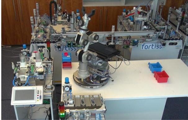
(a) We evaluate our robot task planner on a Robotino mobile platform with a Katana 5-DoF manipulator in a factory setting.
