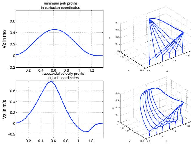
Fig. 2. Left: examples of the robot velocity over time for each condition (top: minimum jerk, bottom: trapezoidal). Right: corresponding trajectories of the robot gripper in Cartesian space for the different six cube positions. The pre-defined hand-over position is located in the upper left part, the initial waiting position in the upper right part. The robot gripper moves from the initial waiting position to one of the cube positions (bottom positions) and from there to the hand-over position.
