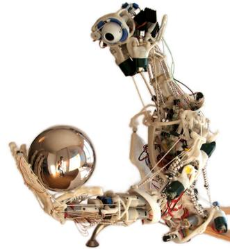
Fig. 1. ECCE, a so called anthropomorphic robot, is the platform for the work presented here. In this type of robot not only the outside of the human body is copied but also the inner structures, like bones, joints, muscles, and tendons.
