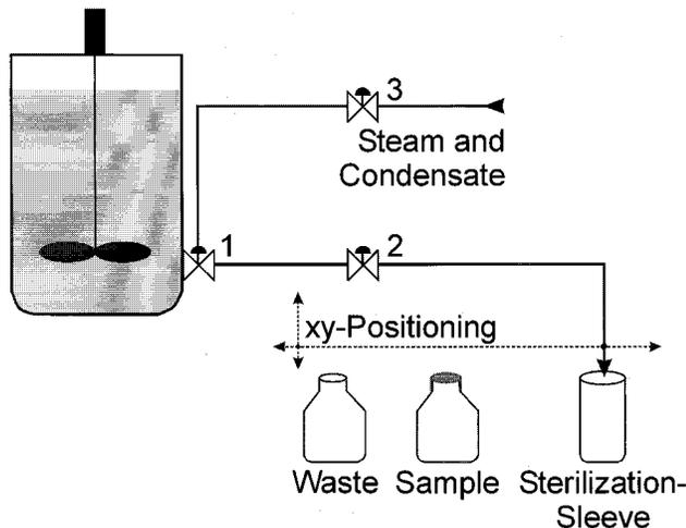
**Figure 2.** Diagram of the steam sterilizable sampling device. The sampling valve (1) is inserted into the bioreactor vessel. Steam sterilization is done via valves 3 and 2. The *xy*-robot places the needle into the sterilization sleeve, waste, or a sample tube. The sample tubes are covered by a septum to ensure aseptic aerosol-free sampling. Using the computerized sampling device the number of samples and the volume are variable.
