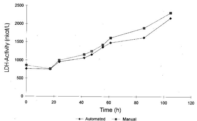
**Figure 5.** To reviewing possible cell disruption caused by the automated sampling device, the LDH-activity was determined. Comparison of manual and automatic sampling during the 20 L hybridoma cultivation the automatic sampling shows a slightly lower activity, which means that there is no cell disruption during automatic sampling.
