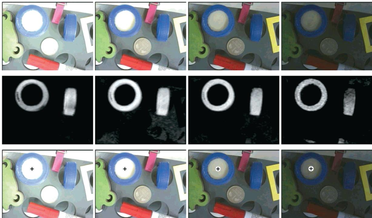
**Figure 8.** Illumination tolerance. The columns from left to right show the original image, the distance measure, and the recognized objects of an overexposed, a normally exposed, and two underexposed situations. In each situation the tube is correctly recognized.
