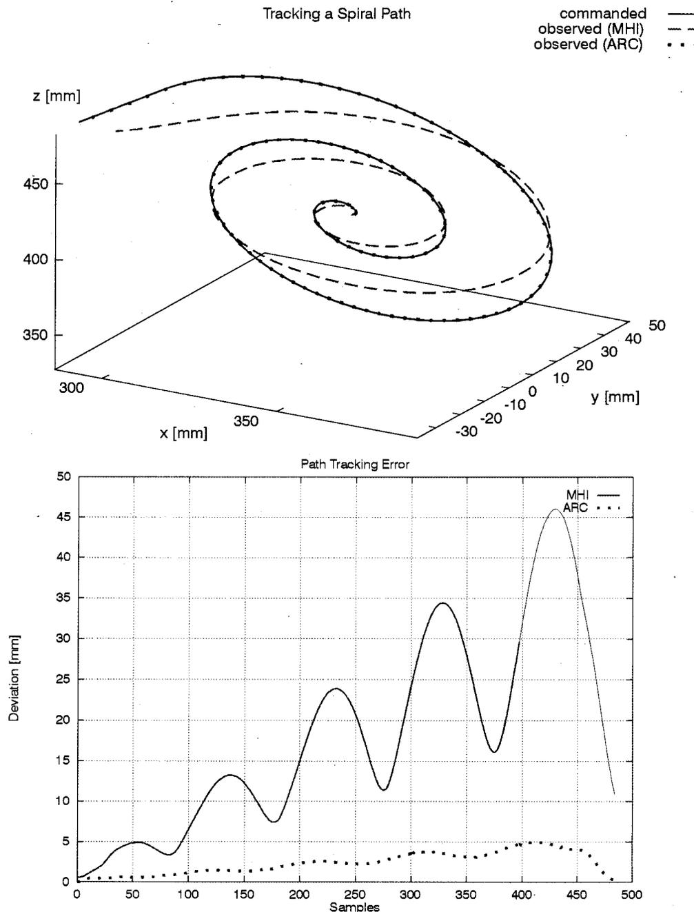
**Figure 6.** Path tracking accuracy. The upper figure shows the commanded and observed path for a sample motion when controlling the robot via the original MHI hard/software and RCCL using the ARCNet interface (ARC). The lower figure shows the path error for both cases; the error has been reduced by 1 order of magnitude.
