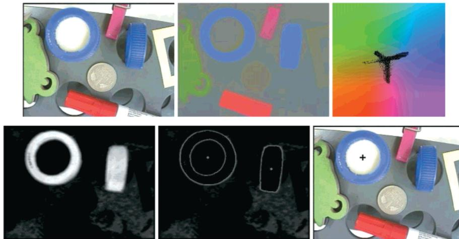
**Figure 7.** Color-based object recognition. The images from the upper left to the lower right show (a) the original image, (b) the color image, (c) the color distribution, (d) the distance measure computed from that distribution, (e) the filled distance measure, and (f) the recognized objects.
