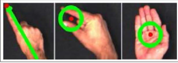
Figure 4: Typical results for the gestures recognized by the JAST vision system. Currently the vision system only interprets the above shown gestures classes.
