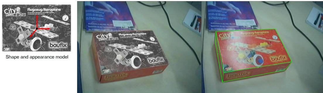
Figure 11. Template-based tracking by Mutual Information maximization.
