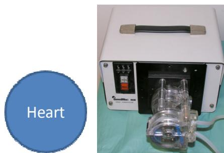
Figure 4. Roller pump (Ismatec BVP) representing the heart
